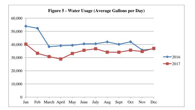
Considering that the average daily usage in 2017 was approximately 34,701 gallons per day, or 173 gpd per household, the pumping system has more than adequate capacity given the current water withdrawal permit to allow for some additional flexibility. Yet, although there is adequate water capacity, one significant problem is the current supply infrastructure and whether it could support any increase in flow that would occur with additional residential development.
